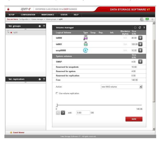
Next, using the "Volume Manager" function you can add a disk volume to a new LV or increase the size of existing LVs (you cannot decrease LV size). To set the needed LV size, just use the scrollbar. On the right side of the scrollbar you will find a counter of available
