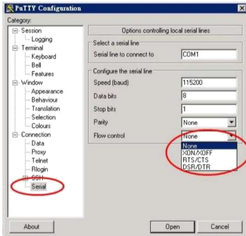
Figure 109: The Procedures of Setup Serial Console by PuTTY_2
