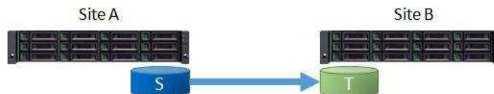
Figure 62: One-Directional Remote Replication
