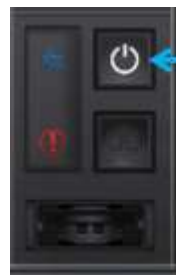
Figure 50: Power off the System by Power Button
