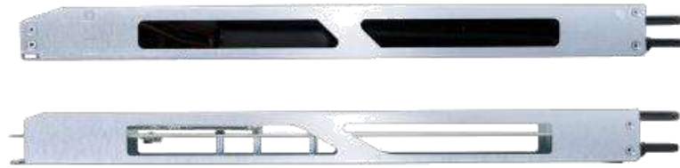
Figure 14: The Cache-to-flash Module – BBM (Battery Backup Module) Pack
