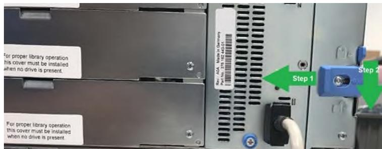
5. Disconnect and completely remove the expansion interconnect cables from the Base Module and from the adjacent modules. Removing the expansion interconnect cables completely prevents damaging the cables when moving the module in and out of the rack.
