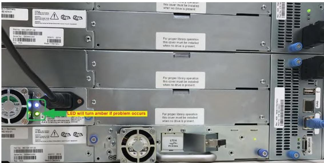
2. Unplug the AC power cord from the power supply you are replacing.
