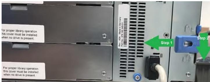
3. Go back to the front of the library, use a Phillips #2 screwdriver to loosen the captive screws fully on the module to be removed and slide the module out of the rack
